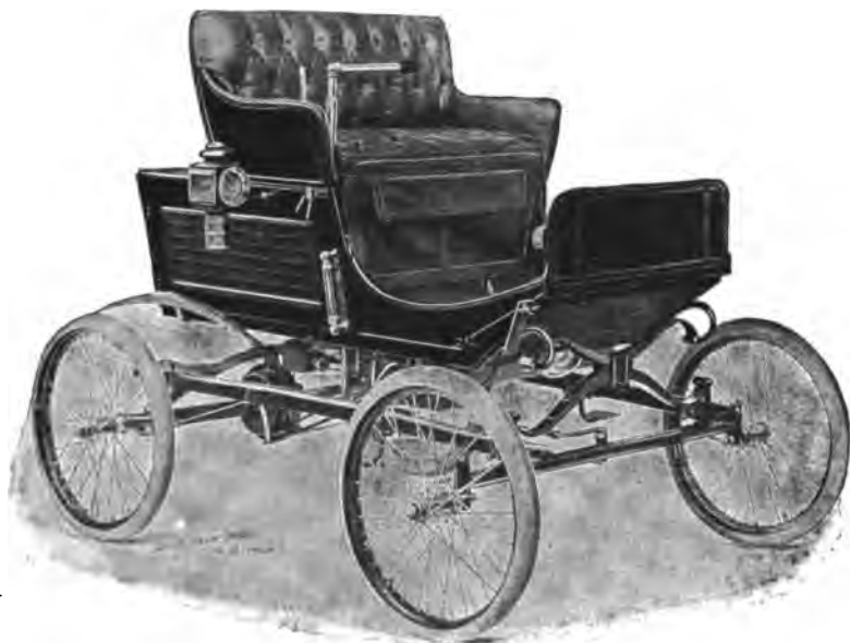
FIG. 82.—A Stearns Steam Runabout, showing side steering lever, solid underframe and the method of arranging the springs.
